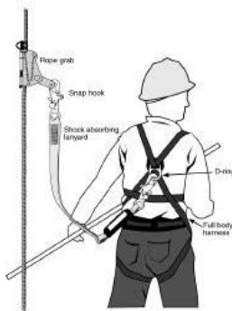
Vertical lifelines are designed to be used by only one person and with a rope grab.
