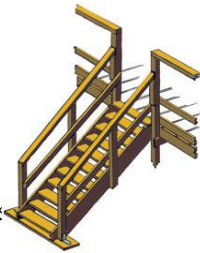
A temporary stairway with handrails
