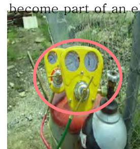
Gas gage protection
