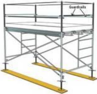
This is an example of a metal guardrail system.
