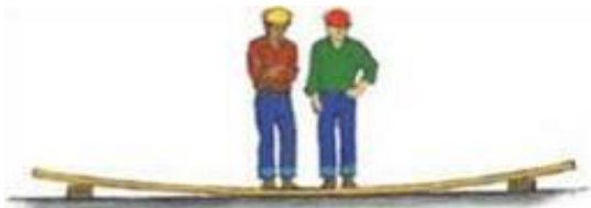
To test a plank, have two workers stand on the centre of it.
