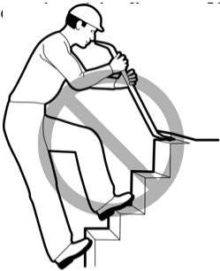
Pry From A Stable Position
