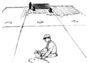
The flotation compartment of a barge is a confined space that may not have enough oxygen to sustain life
