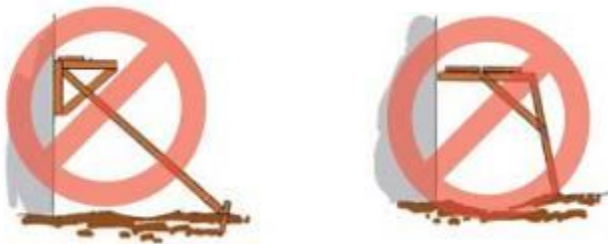
The use of shore scaffolds (top) or lean-to scaffolds (bottom) is PROHIBITED.
