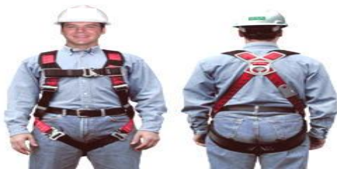
This is a full body harness worn to arrest falls. Note that the D-ring is located between the shoulder blades.
